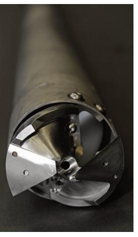
diameter drills with a hollow core that enables samples to be collected in the bore of the drill. This is a slow process that takes months to get to the necessary 3km depth of one million year old ice. So choosing a site that has a relatively high geothermal temperature could spell disaster and ruin many months of effort.
