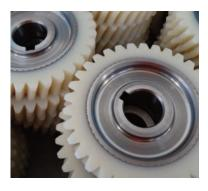
steering system. Nylacast's worm wheel is made from a combination of polymer and steel. The steel inner hub provides dimensional stability and strength, while the outer ring is made from a custom formulated grade of copolymer 6.12 developed by Nylacast's R&D department.
