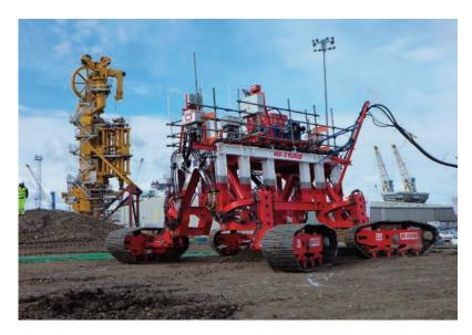
for inter-array cable burial. A four track crawler system would provide better manoeuvrability than two track, skid-steer vehicles, while it's patent pending levelling system enables vertical trenches to be cut whilst the device is on slopes of up to 20°.
